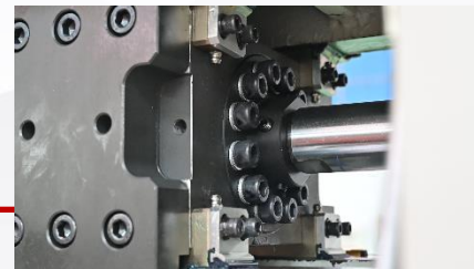
Check the fixing screws at the end of the piston of the stretching cylinder
