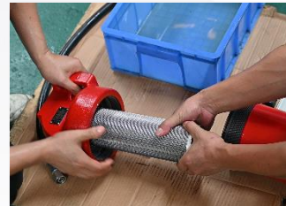
(5) Take out the filter element
