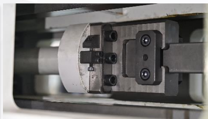
Check the fixing screws of the connecting part between the mandrel-pulling cylinder and the mandrel
