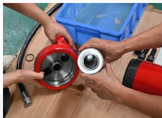
(6) Change the filter element
