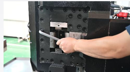
Check the fixing screws of the jaw cover plate
