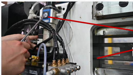
Check whether there is lubricating oil sprayed at the mandrel and whether the pressure gauge changes.
