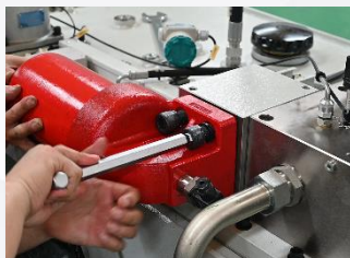
(8) Reinstall the filter element
