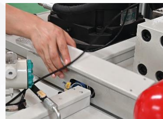
(9) Install the white cover plate back
