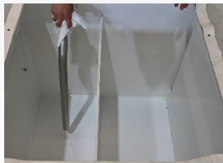
(3) Use lint-free cleaning cloth to wipe the interior of the oil
