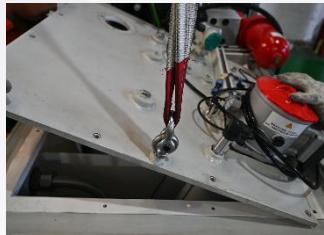
(2) Remove the top of the oil tank
