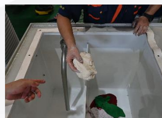
(4) Use a flour dough to clean the dust, debris and other impurities in the corners of the oil cylinder
