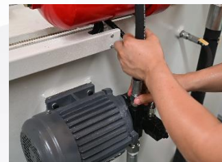
(10) Install a new oil inlet pipe for motor cooling
