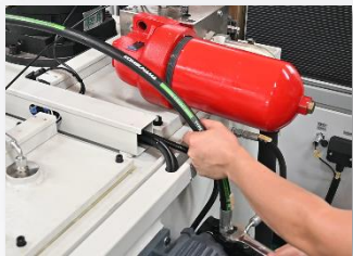
(1) Remove the oil inlet pipe for motor cooling.
