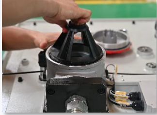
(2) Take out the filter element
