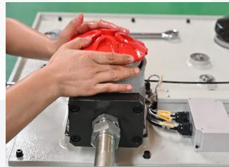
(7) Tighten the red nut
