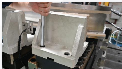
Check the fixing screws of the front pressing and cutting device on the tooling
